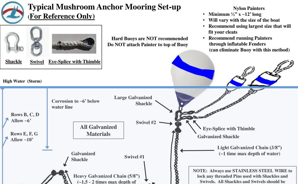
NOTE: Mushroom anchor must be worked into bottom for maximum holding power.
